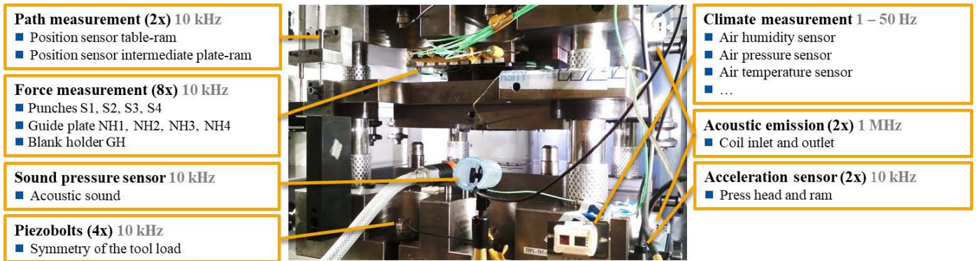
Figure 5: The fineblanking tool displayed is equipped with various sensors to acquire sensitive process information. All the information generated by the sensors in the above figure are not transferred via the SPS-bus system, but acquired with additional measuring equipment.
